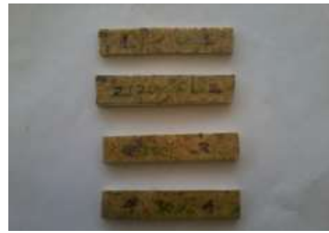
Fig.27 Izod impact test specimen ASTM D 256
