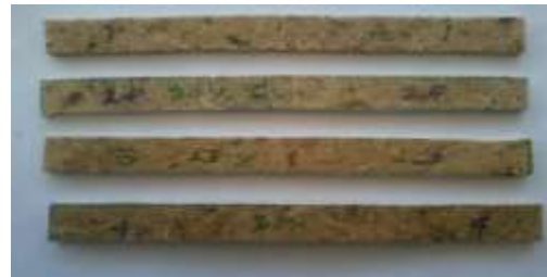
Fig.22 Flexural Strength Test specimen
